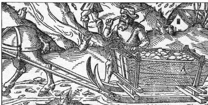
Fig.17 Illustration from 'De Re Metallica' of a sledge used in Iron mining.
